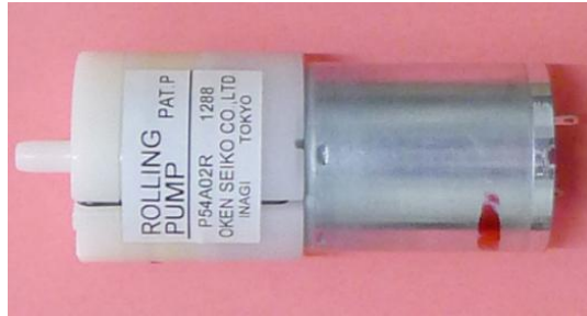
Figure 3.7 : Air pump motor (P54A02R)
