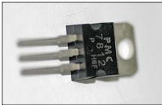
Figure 3.16: Popular three pin 12 V DC voltage regulator IC.
