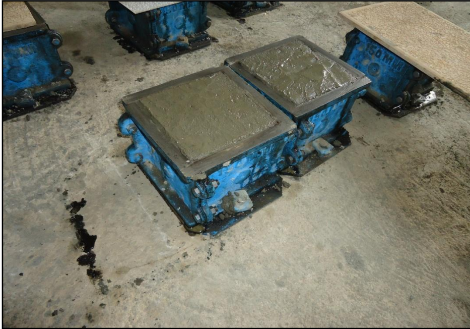
Photo (6): Concrete specimens after casting
