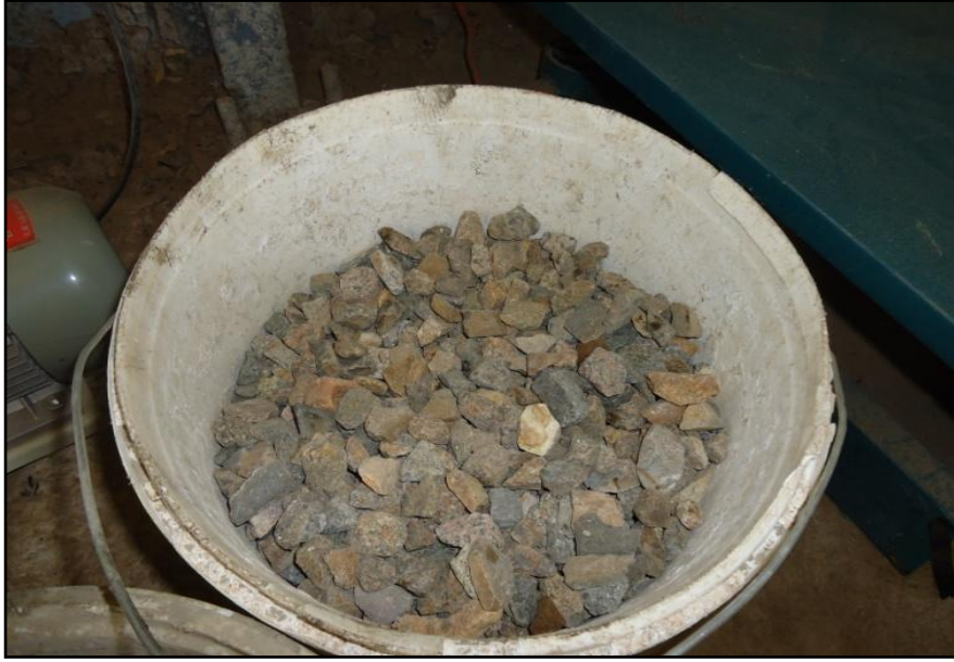
Photo (4): Crushed stone for concrete
