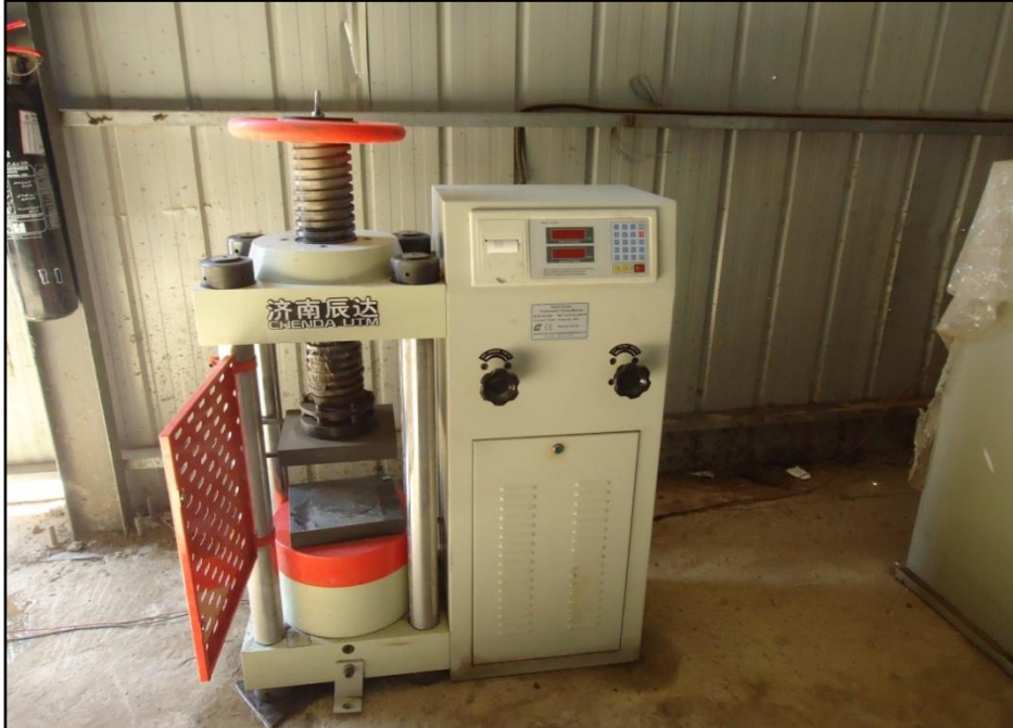
Photo (7): Compressive strength testing machine
