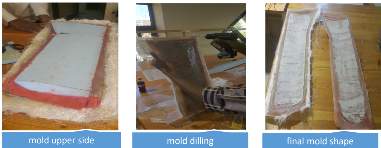
Figure 4-2 wing mold manufacturing
