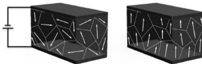
Figure 2-5 electrical force effect
