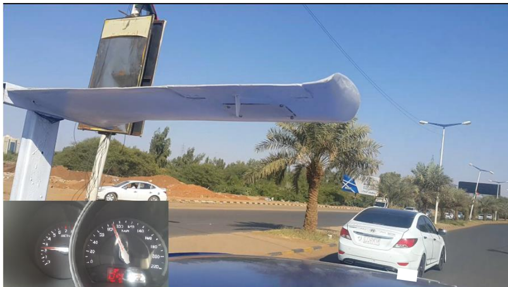
Figure 4-11 wing testing on the charging speed
