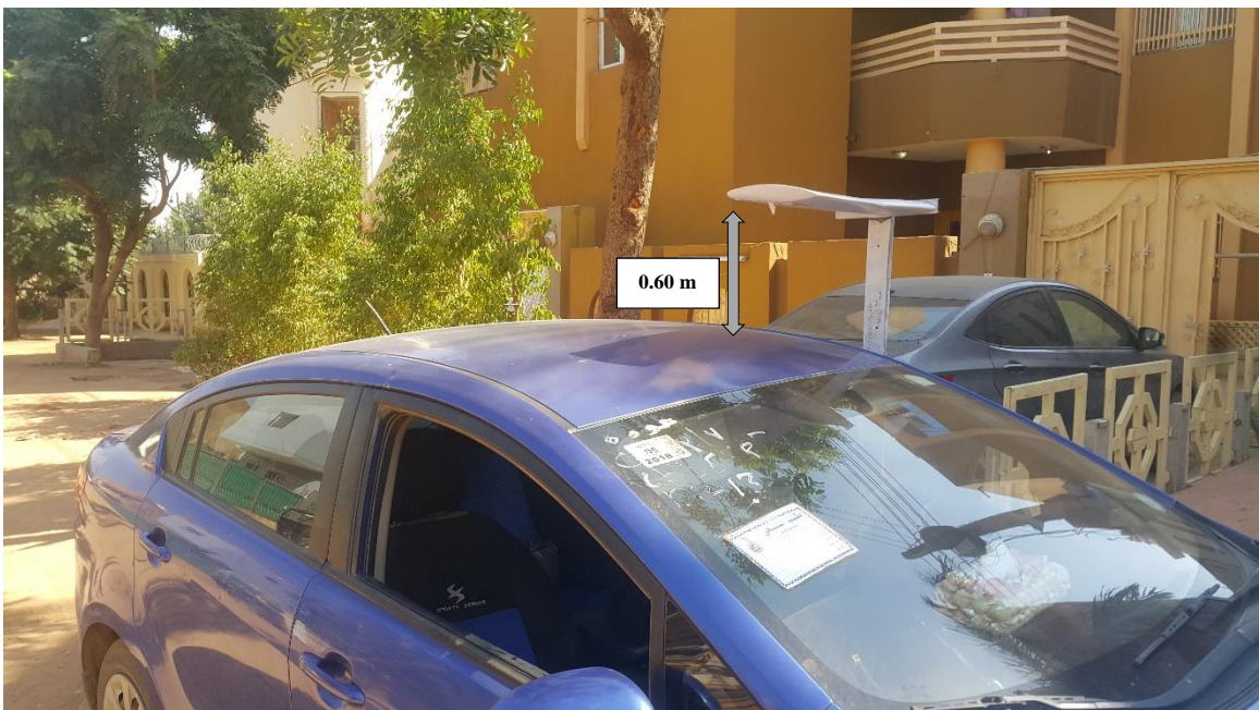
Figure 4-9 Car-mounted wing test rig
