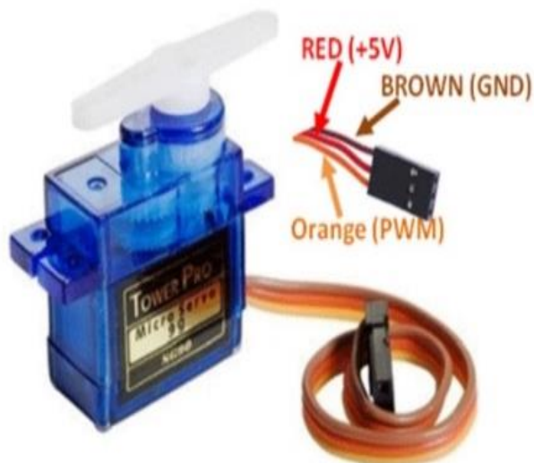
Figure 4-5 micro servo motor
