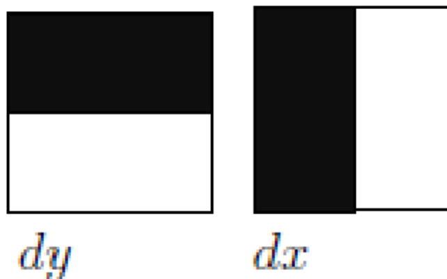
Figure 3.5: The wavelets response. Black and white areas corresponds to a weight-1 and 1 for the Haar kernels
