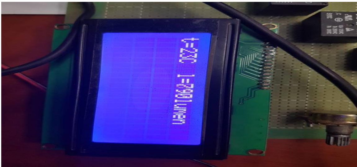
Figure 4.11 Temperature and light values in manual mode
