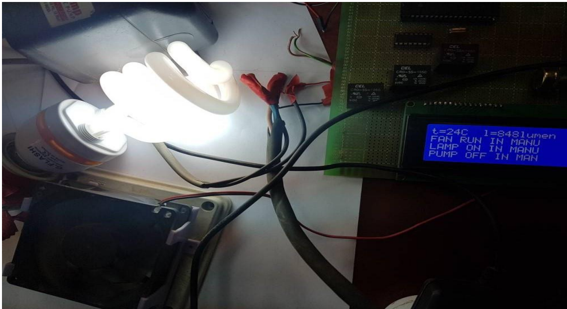
Figure 4.14 fan and lamp run but pump off
