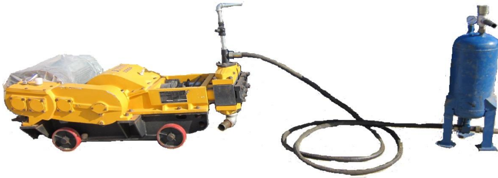
Figure 3-7: 3 SNS grouting pump and pressure control device
