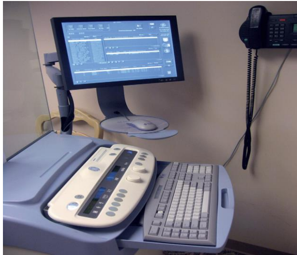
Fig: 2.16 The acquisition workstation (AW) consisting of a computer, computer monitor, keyboard, mouse or trackball, and software specific to the full-field digital mammography (FFDM) manufacturer.
