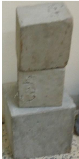
Figure 3.6: A picture of cement mortar cubes.
