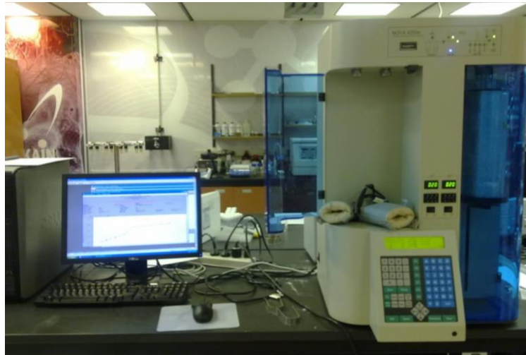
Figure 3.7. The Brunauer–Emmett–Teller (BET) surface area analyzer King Fahad for Minerals and Petroleum University, Saudi Arabia.
