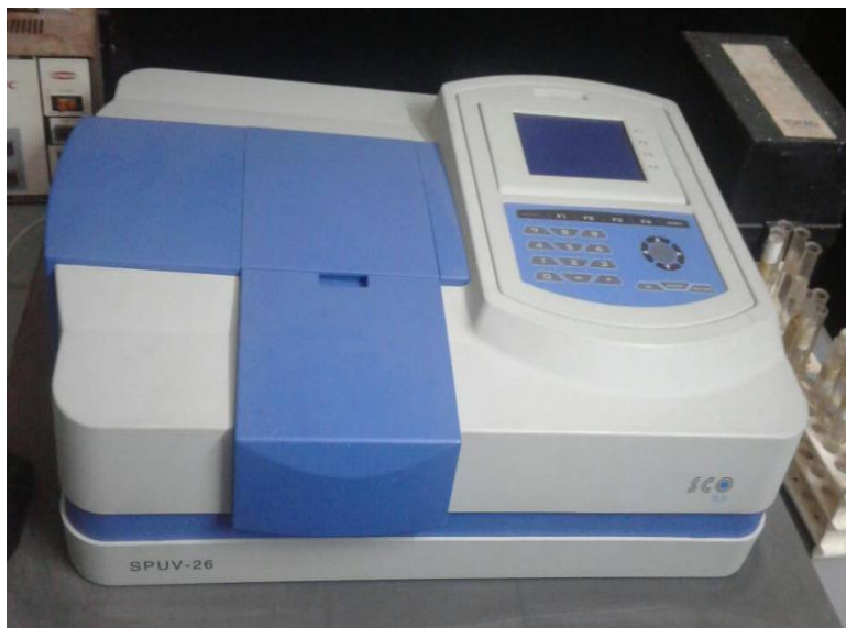
Figure 3.9. The ultra-violet- visible (UV-Vis) spectrometer, Sudan University of Science and Technology, Sudan.
