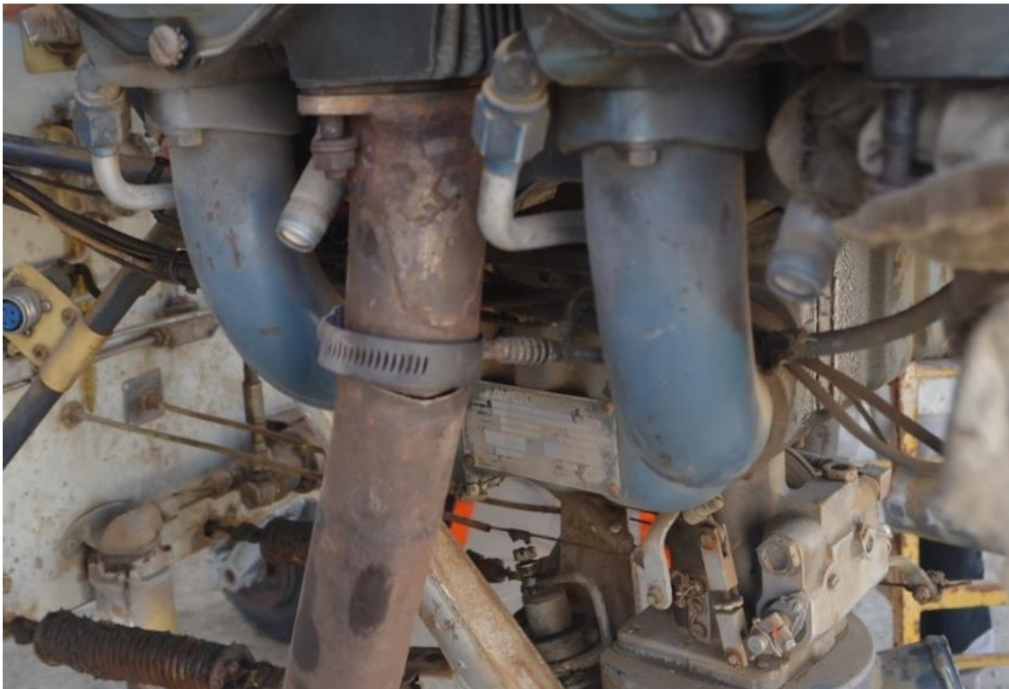
Figure 1.2: UTVA 75 exhaust crack
