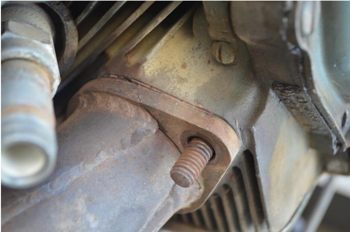
Figure 1.1: Utva 75 exhaust crack
