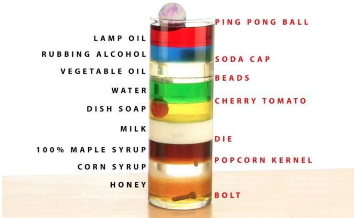
Figure 2.5 comparison between the density of fluids and solids
