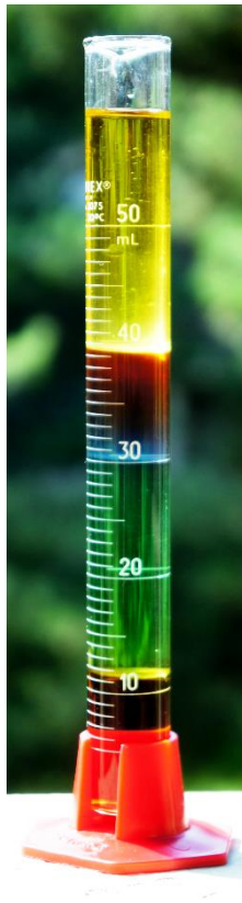
Figure 2.4 cylinder with colored fluids with different densities
