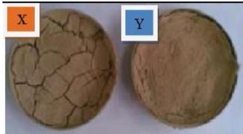
Fig. 2.5 Aridness cracking (X) unreinforced sample (Y) reinforced sample [46]
