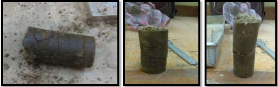
Fig 3.14 segregation and cracks on fiber glass samples
