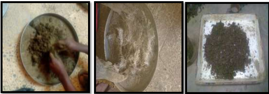
Fig 3.13 Plain Soil mixed with fiber glass, PET Strips and cement waste
