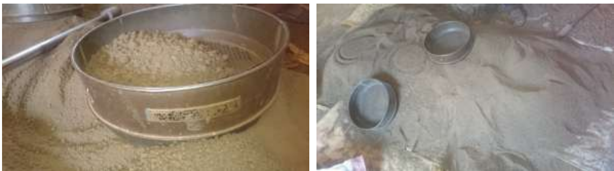
Fig 3.2: Clay soil preparation (air dried sieve no 4)
