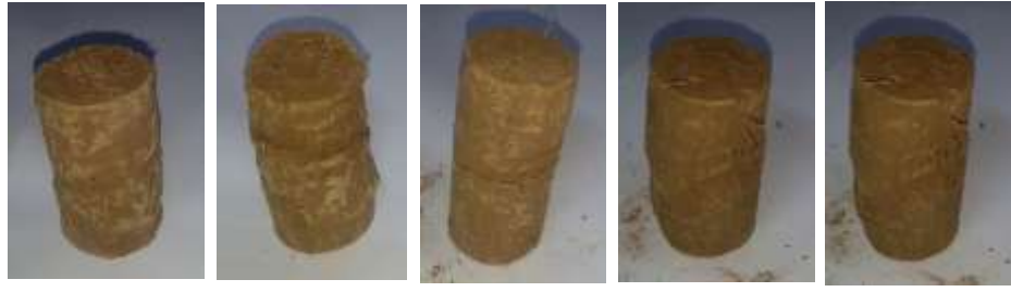
Fig 4.70 Shape of failure on soil Reinforced by fiber glass waste (Cracks failure)
