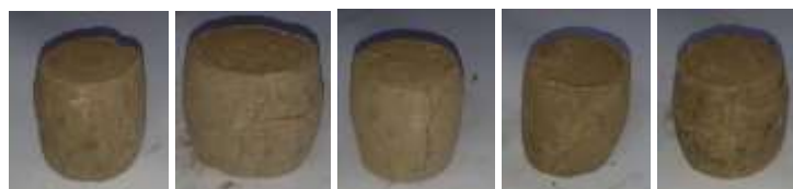
Fig 4.51 Shape of failure for soil treated by cement waste (buckling and cracks)
