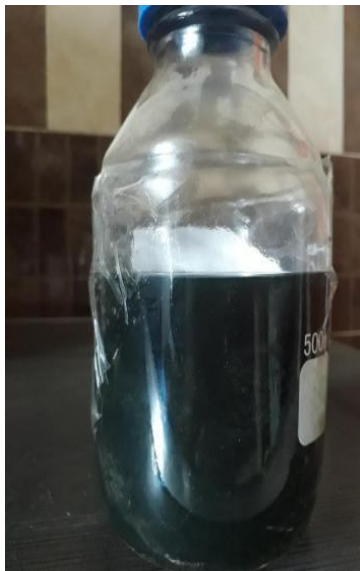
Figure (4.12): Oil from mixture (1:1:1) of PP/HDPE/LDPE
