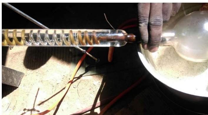
Figure (4.1): oil stuck inside the condenser
