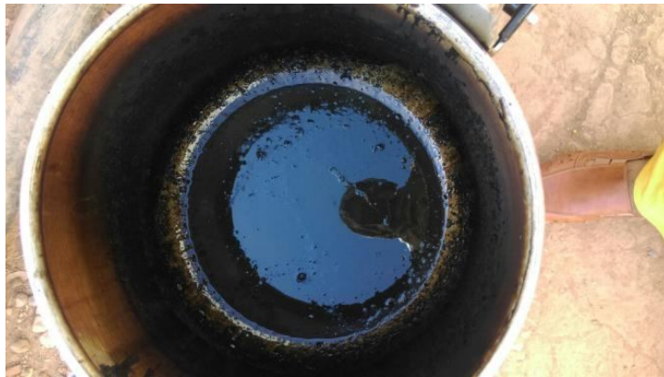
Figure (4.5): HDPE sludge remain in the reactor
