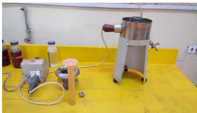
Figure (4.16): The kinematic tester
