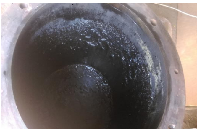
Figure (3.7): Pyrolysis Residues for HDPE using V1 reactor
