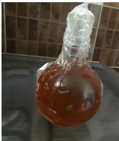
Figure (4.14): Oil from LDPE wax after second stage pyrolysis
