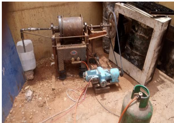
Figure (3.4): Horizontal reactor V3
