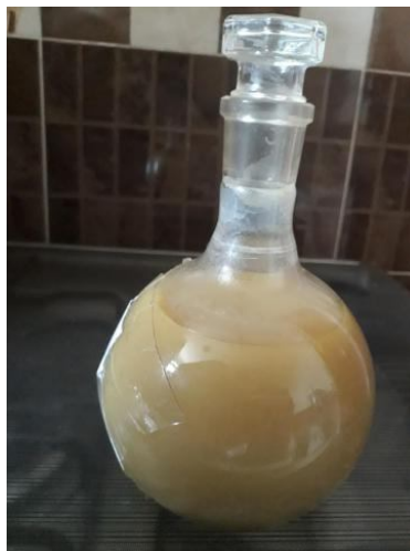
Figure (4.11): Wax from mixture (1:1) LDPE/HDPE
