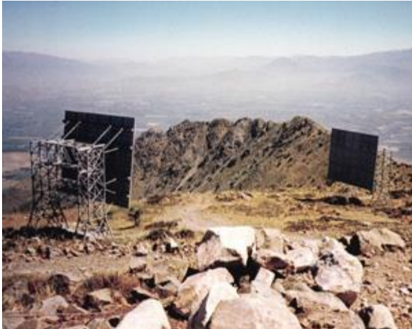
Figure 2.4. Passive relay station (Plane reflectors)
