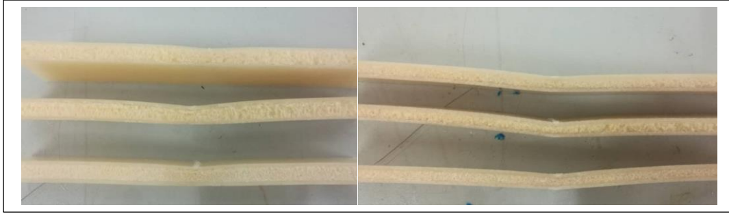
Figure 4-5: Shows cross-sectional view of specimen with 3 and 6 mm core thickness pending test.
