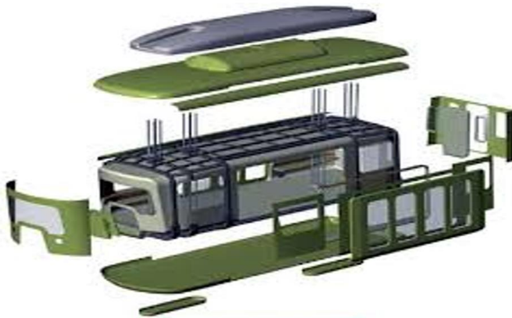
Figure 1-1: Module composite sandwich car body structure
