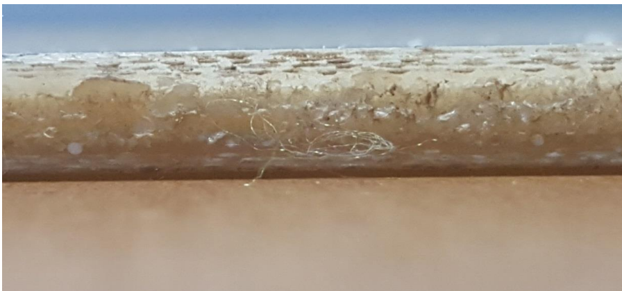
Figure 3-4: Composite materials sample with 3mm core thickness.
