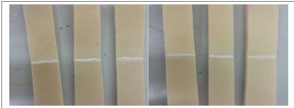
Figure 4-4: Shows surfaces of specimen with 3and 6 mm core thickness pending test.
