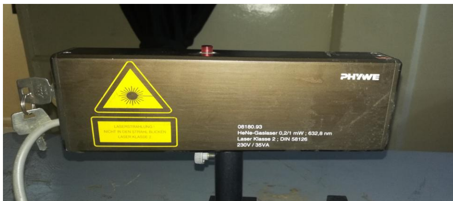
Figure 3.2: He-Ne Laser (632.8 nm, 2 mW)
