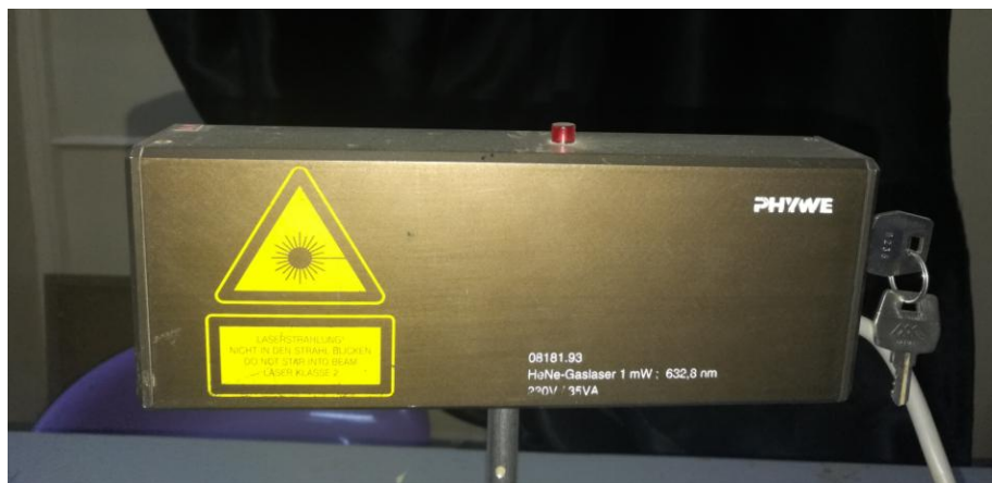
Figure 3.1: He-Ne Laser (632.8 nm, 1 mW)
