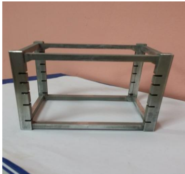
Fig2.4 ISRASAT1 Mechanical Structure Frame
