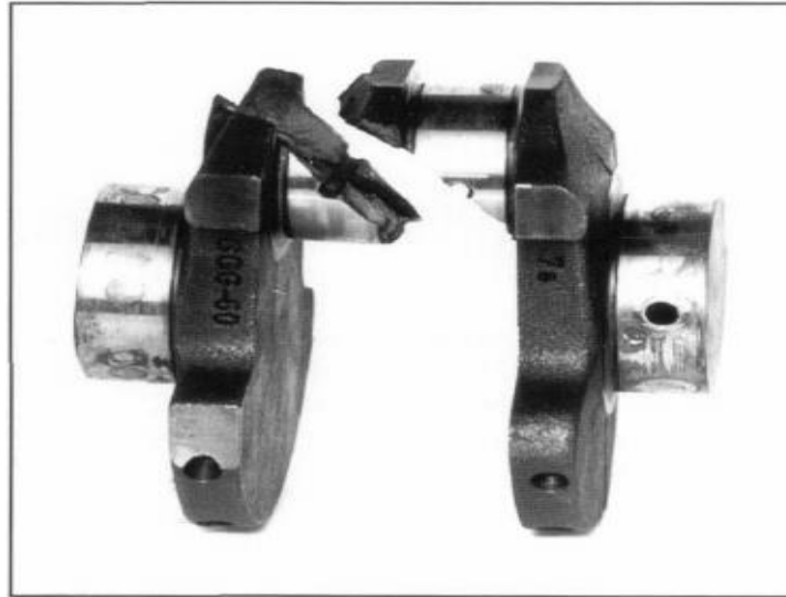
Figure 1-2 Sample failed engine crankshaft (in 45° due to torsional vibration) [12]
