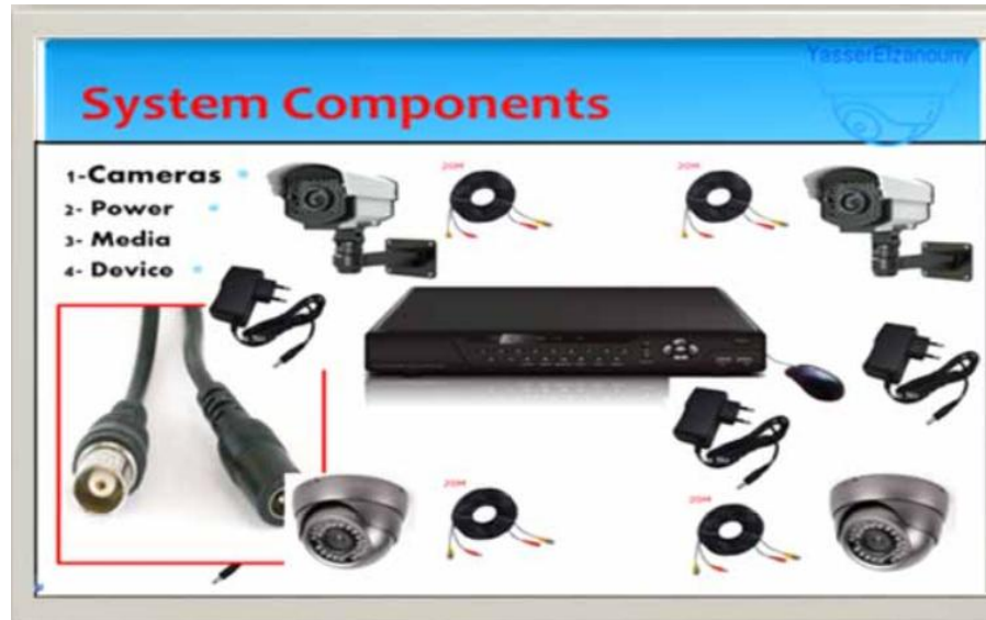
Figure (2. 1): Basic Components of CCTV System[9]
