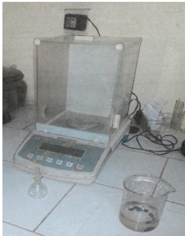
Figure: 3-7 density equipment tests
