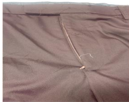
Figure 4.18 More numbers of sewing thread in the product in x_1 factory because the scissors of the sewing machine deactivated
