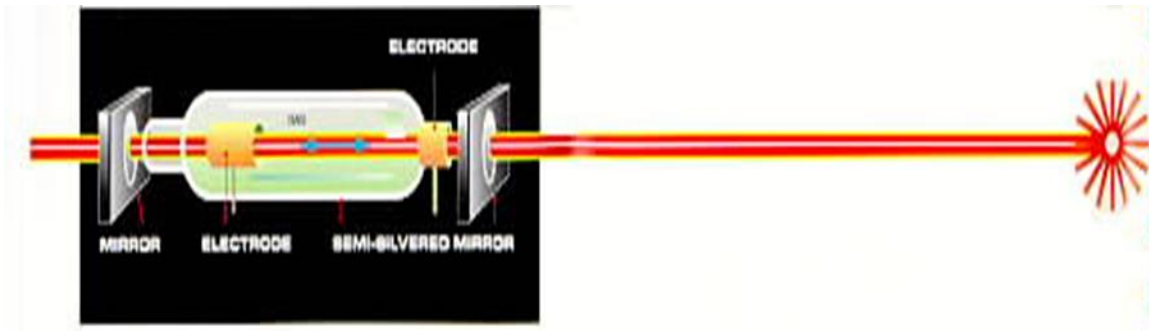
Fig: 2: 1 This picture shows the optical cavity of a gas laser with its totally reflecting mirrored end and partially reflecting mirrored end through which the laser beam is emitted. The energy source (not shown) is called the pump.
