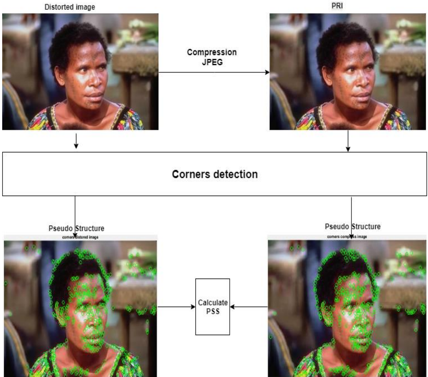
Figure (4.1): A framework of the PRI-based BIQA metric PSS for blockiness estimation to measure similarity for pseudo structures from distorted image and PRI. Circle green denote number of corners.
