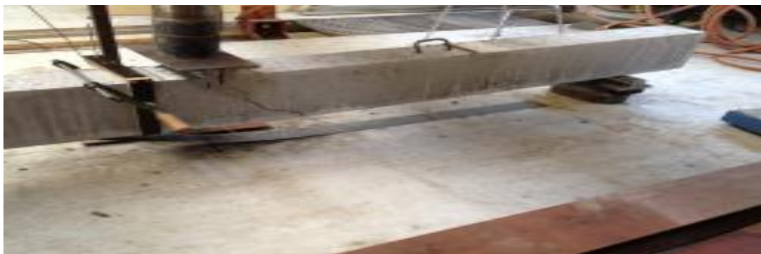
Figure: Crack pattern for de-bonding failure
