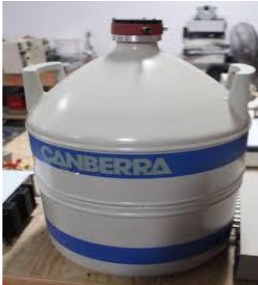
Figure- 3.7 Cryostat Canberra filled with Liquid Nitrogen (LN 2 )
