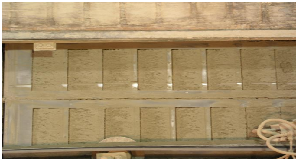
Figure- 3.13 Soft-Mud Process
