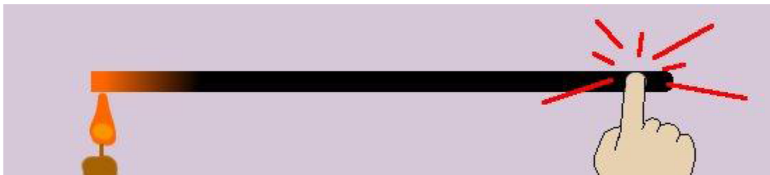
Figure- 2.1: Conduction heat transfer
