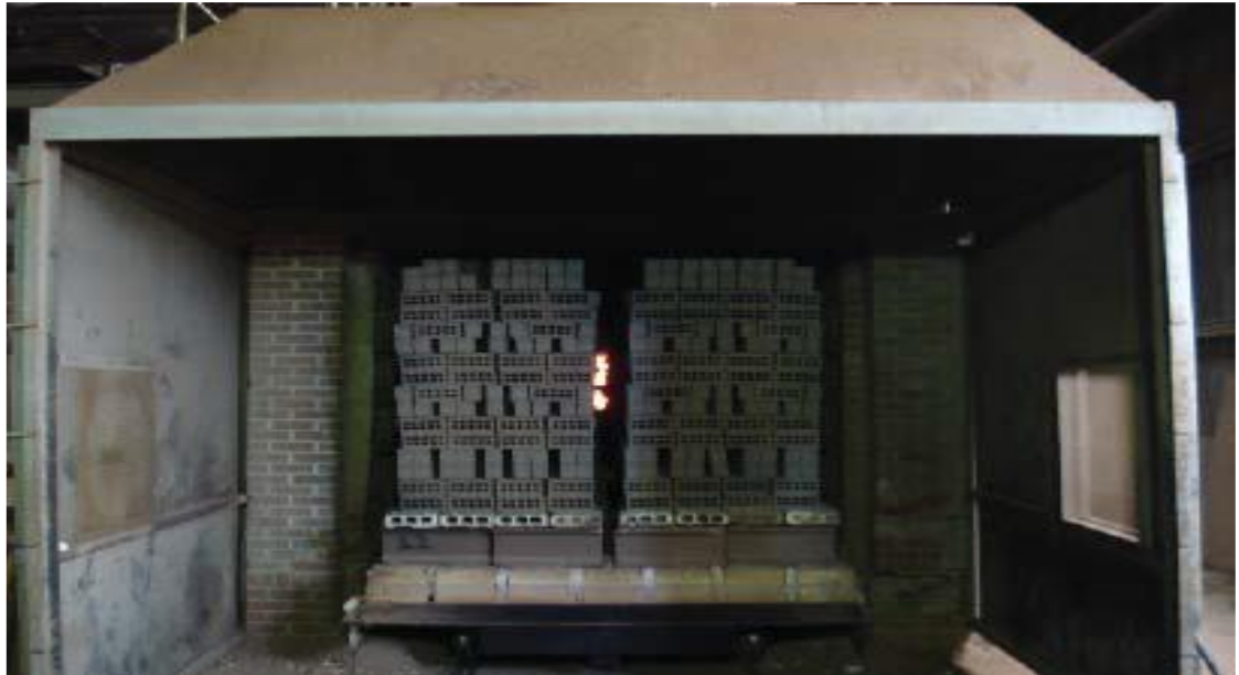
Figure- 3.14 Brick Enter furnace for Firing
