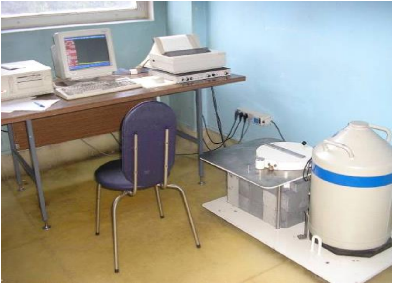
Figure- 3.4 The System used to Analyze the Concentration of Elements by Canberra 35+ Device
