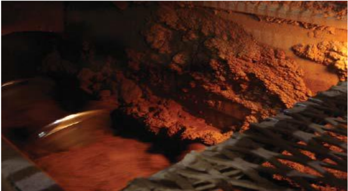
Figure- 3.10 Clay is Thoroughly Mixed with Water in Pug Mill before Extrusion
