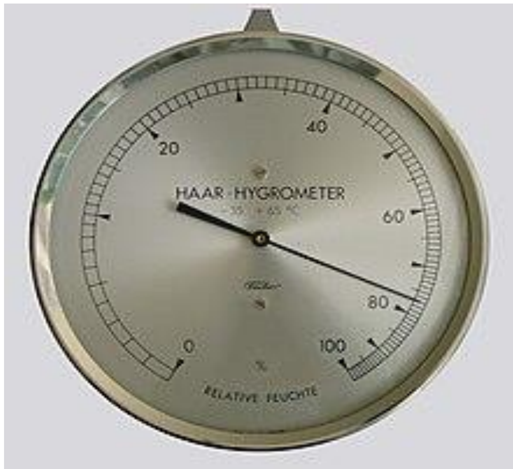
Figure- 3.19 A hair Tension Dial Hygrometer with A nonlinear Scale
