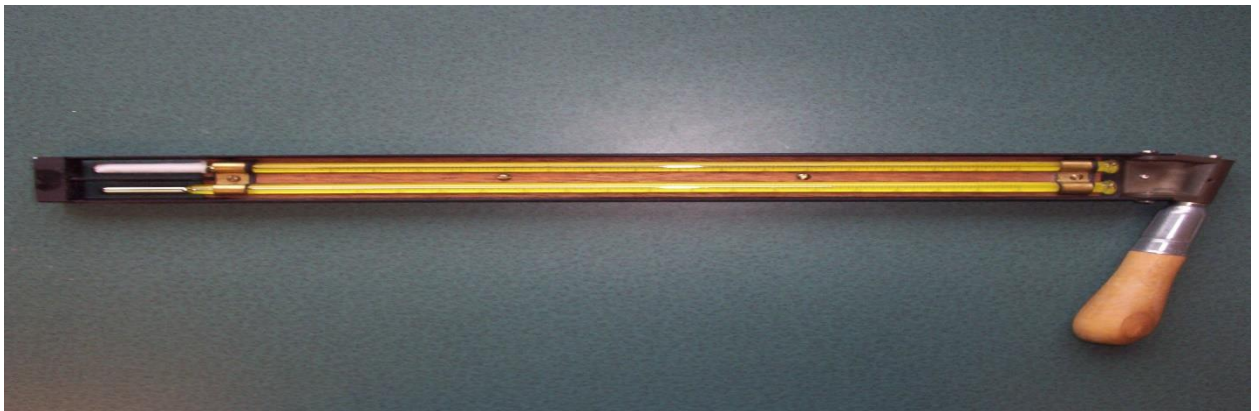
Figure- 3.18 A sling Psychrometer for Outdoor Use
