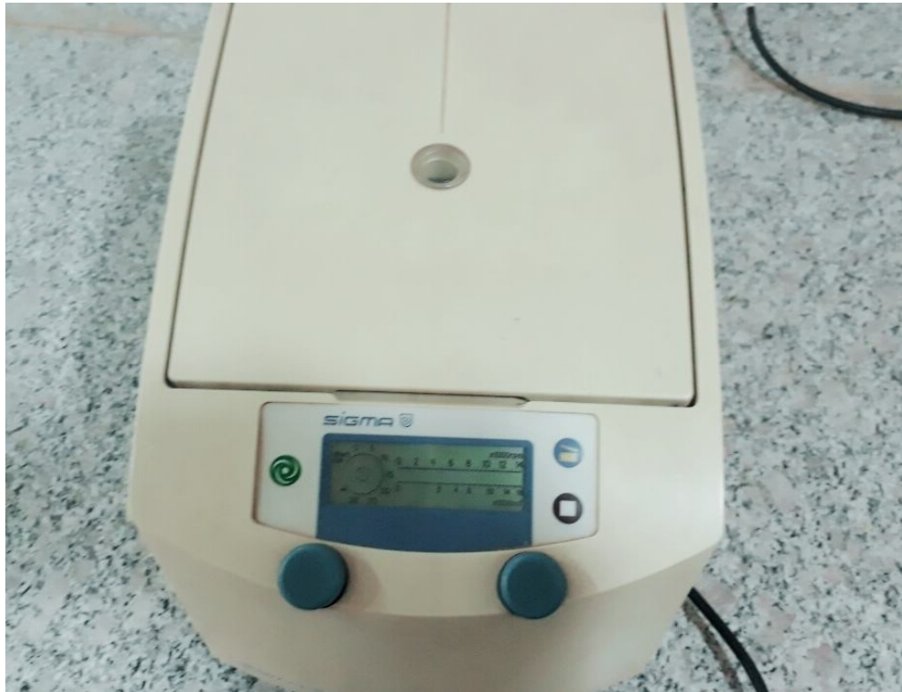
Fig24 : Sigma 1-14 Germany Microcentrifuge Device (In Medical Research lab at Sudan University of Sciences and Technology).
