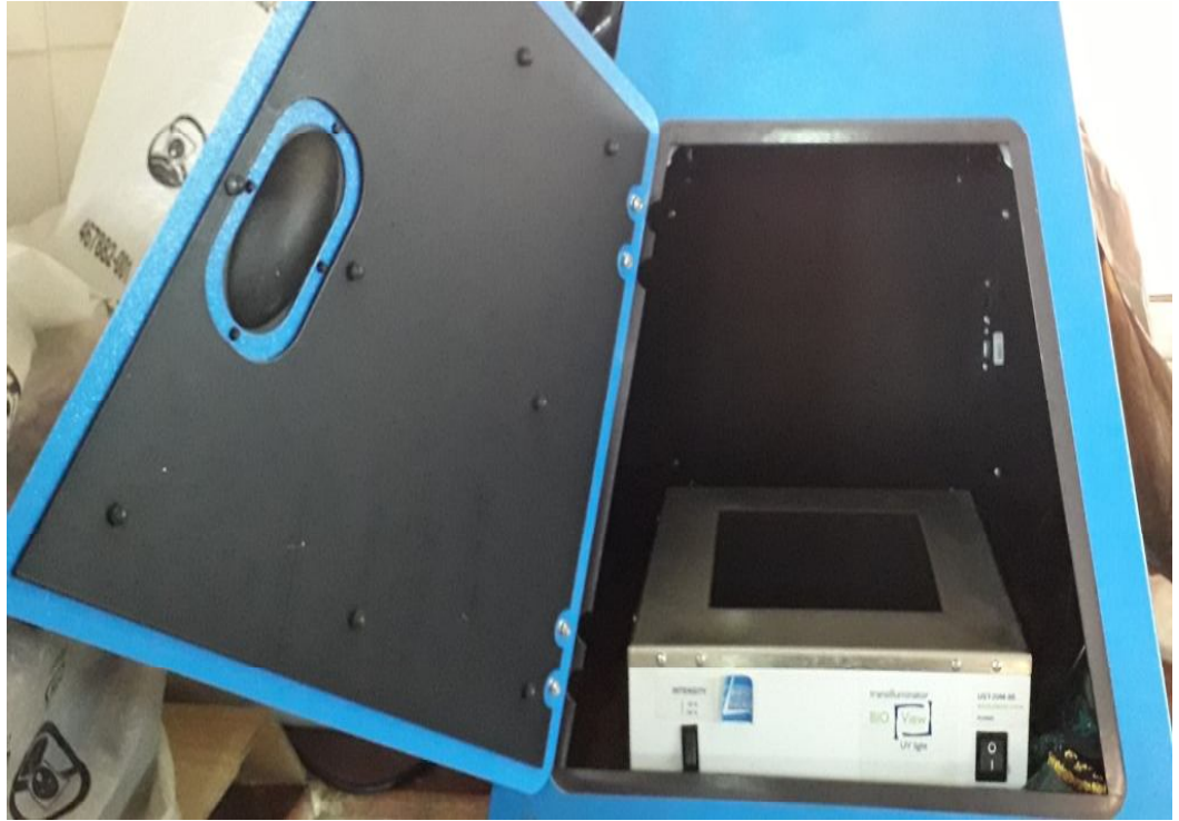
Fig 28: UV Light Transilluminator Device (In Research laboratory College of Veterinary Medicine Sudan University of Science and Technology) •
