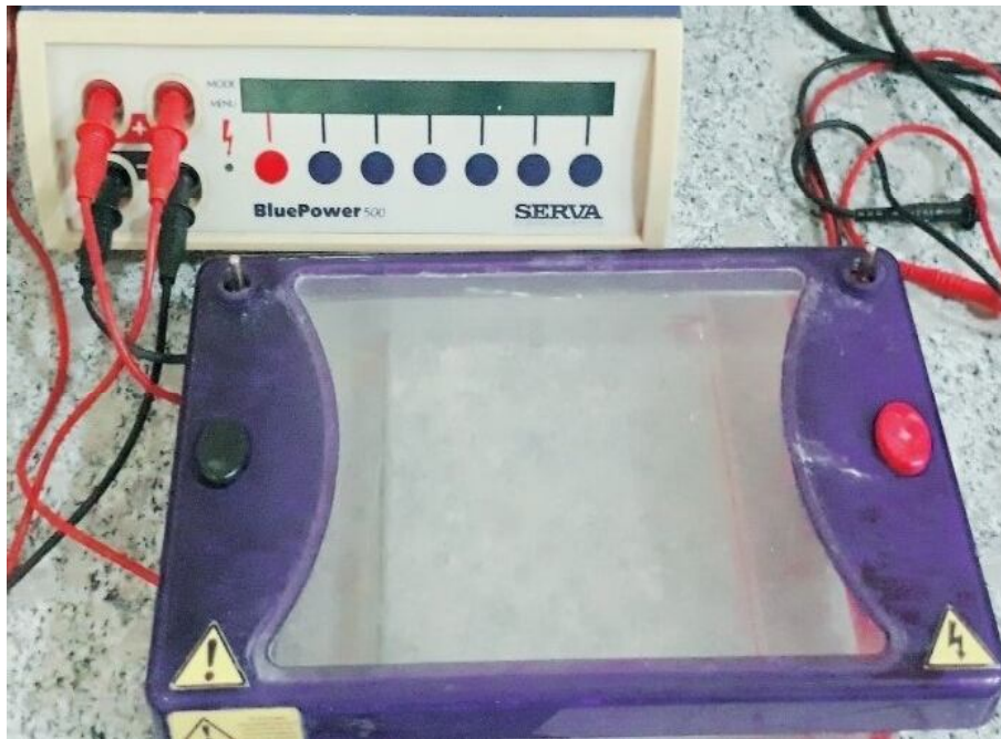
Fig27: Gel Electrophoresis and Power Supply Device(In Medical Research lab at Sudan University of Sciences and Technology).
