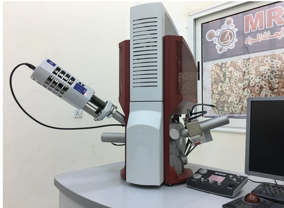
Figure 3.5: A photograph of the FESEM, shown
