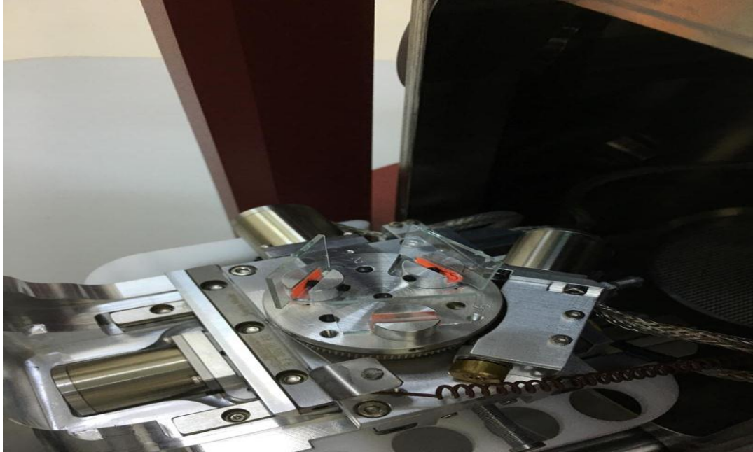
Figure 3.6: FESEM stage and sample holder
