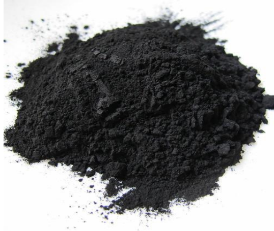
Figure 1.2: Powdered activated carbon (PAC)
