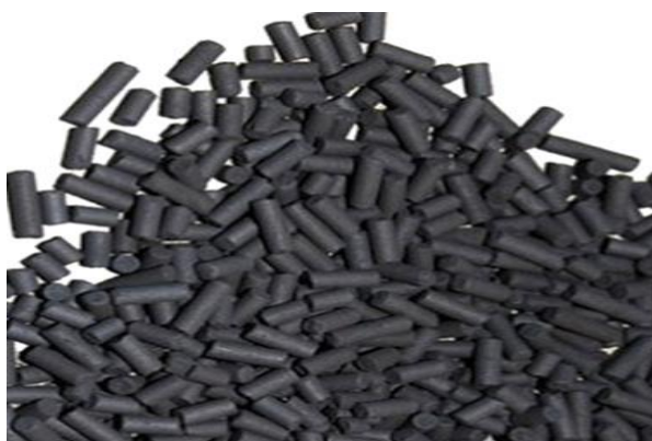
Figure 1.4: Extruded activated carbon (EAC)
