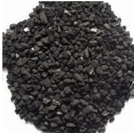
Figure 1.3: Granular activated carbon (GAC)
