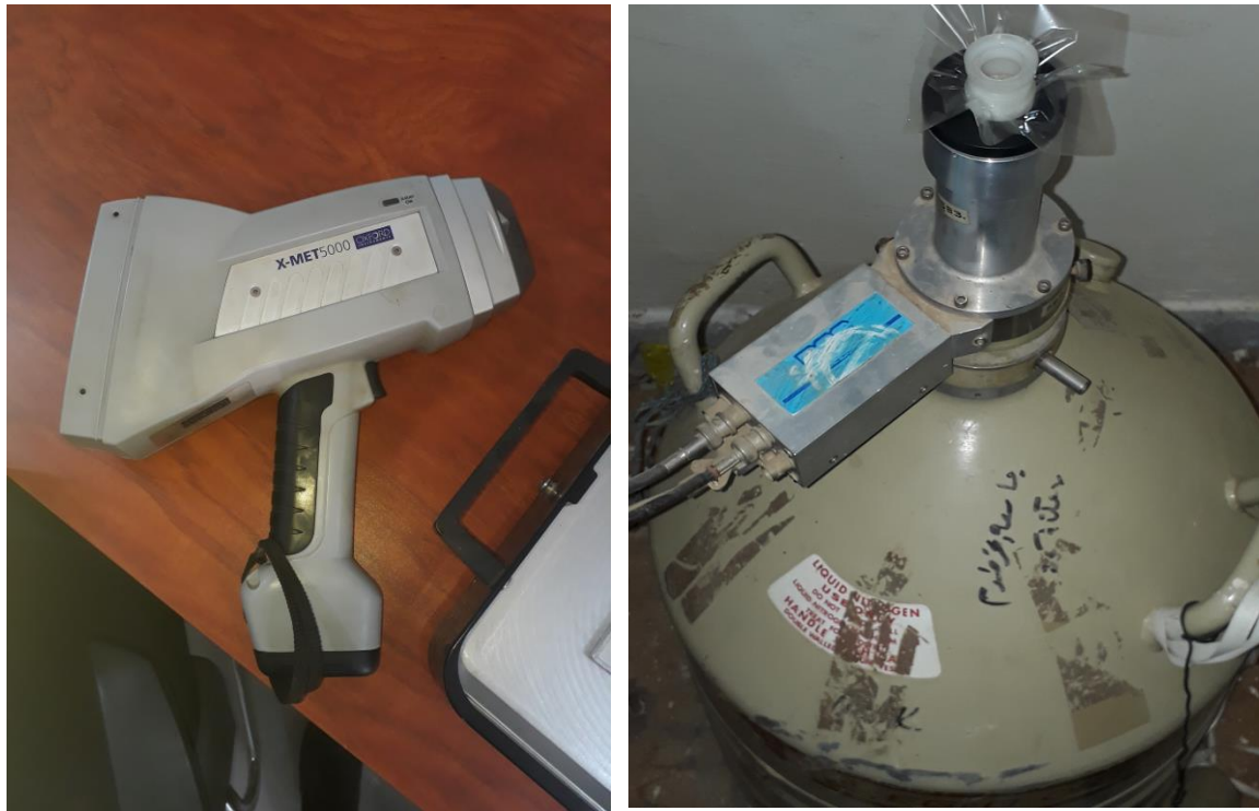
FIG 2.1 shows tow type of XRF used in sample analyzed
