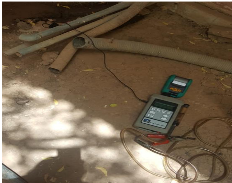
Figure (2.12): Gas analyzer connect to exhaust
