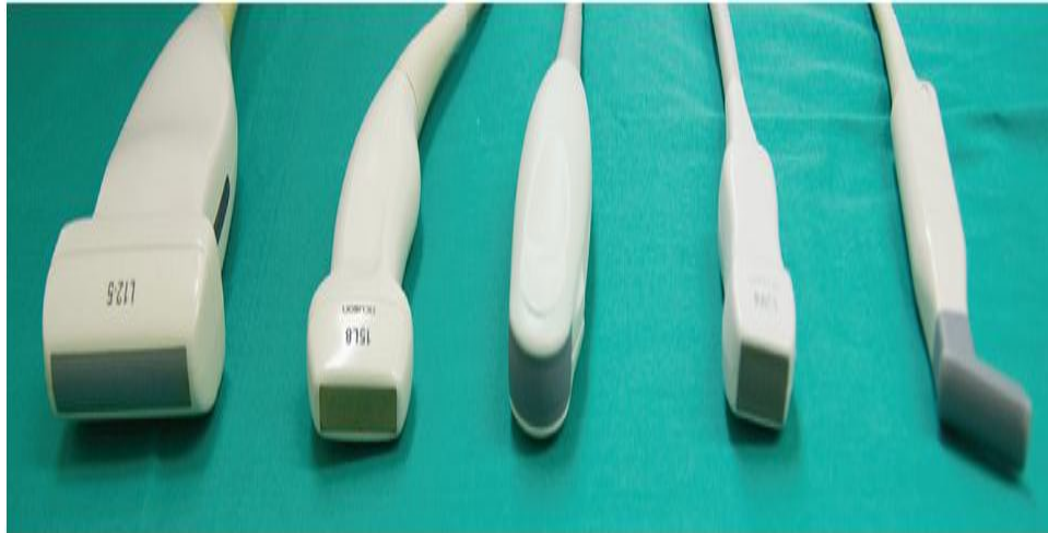
Figure 2.14. Shows Ultrasound transducers for regional blocks. The photograph includes (left to right) broad linear, small footprint linear, curved, sector and hockey-stick transducers. (Andrew, 2013).
