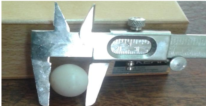
Plate (7a): Measurement of length of egg by vernier caliper
