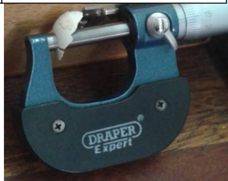
Plate (9): Measurement of the thickness of egg shell by micrometer
