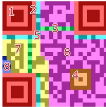
Figure 3.1: Structure of QR Code Version 2
