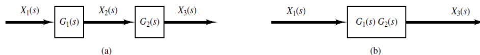
Figure 2-7 (a) System consisting of two nonloading cascaded elements; (b) an equivalent system.
