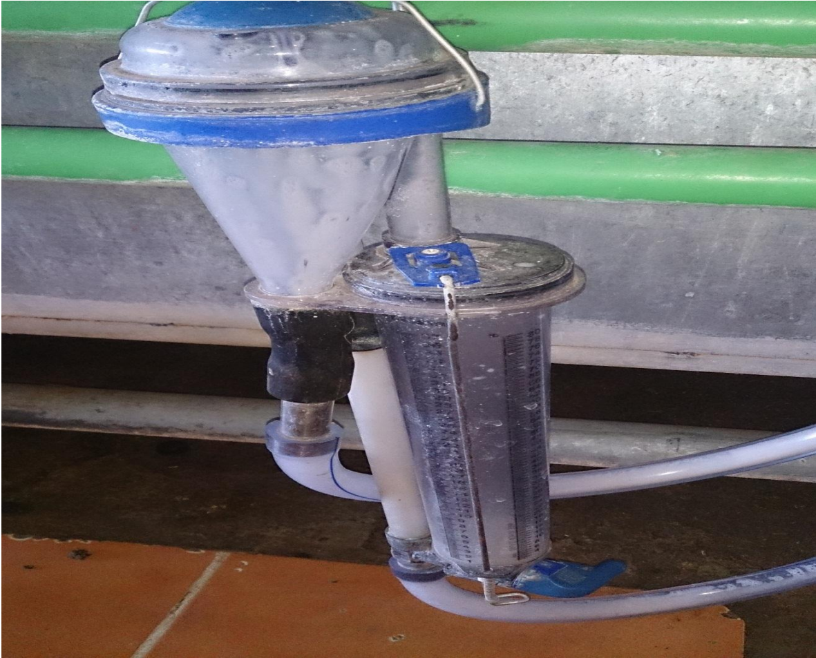
Photo 3.2 cylinders milk yield recorders attached with the milking machine for each cluster. Al-Turath Company – Jeddah. (Musaad M. A 2015).
