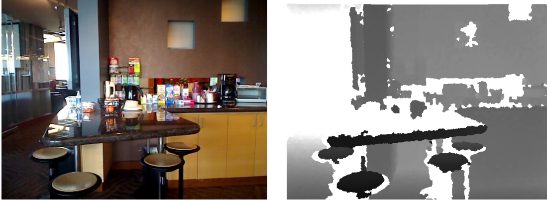
Fig. 2.8 (left) RGB image and (right) depth information captured by an RGB-D camera.
