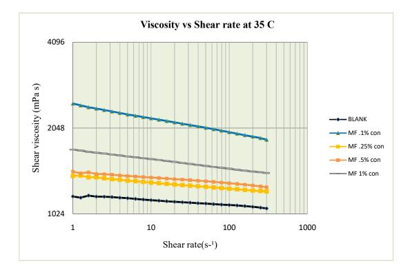
Figure (4-4): Viscosity Vs. Shear rate for sample (1) with different concentration at 35 C.
