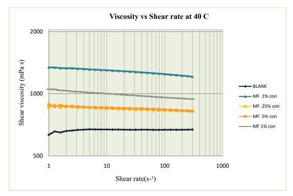
Figure (4-5): Viscosity Vs. Shear rate for sample (1) with different concentration at 40 C.
