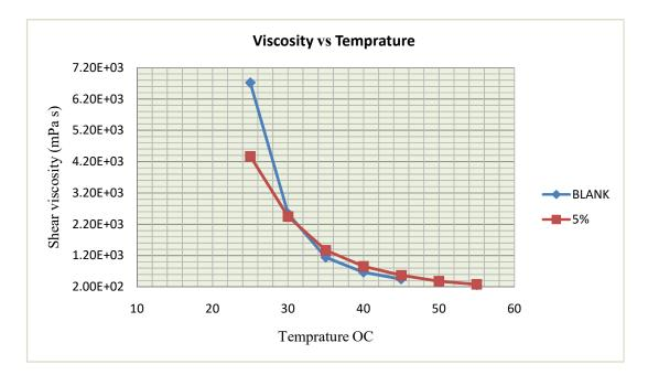
Figure (4-18): Viscosity Vs. Temperature for sample (1) with 0.5% MF concentration.
