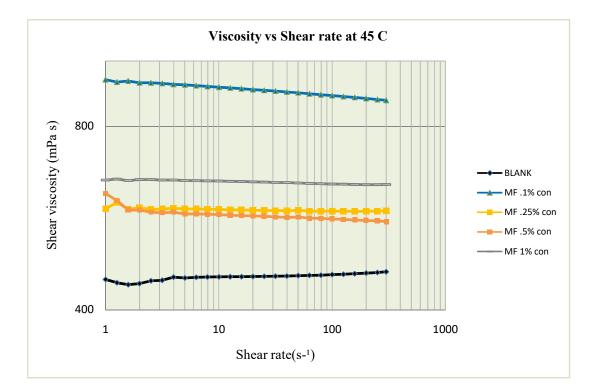
Figure (4-6): Viscosity Vs. Shear rate for sample (1) with different concentration at 45 C.
