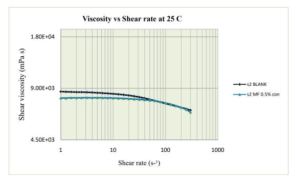
Figure (4-10): Viscosity Vs. Shear rate for sample (2) with 0.5% MF concentration at 25 C.
