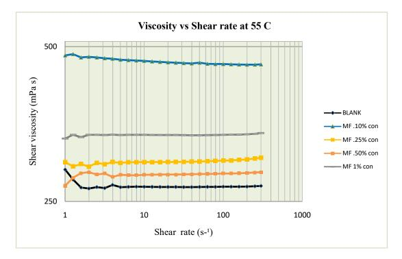
Figure (4-8): Viscosity Vs. Shear rate for sample (1) with different concentration at 55 C.
