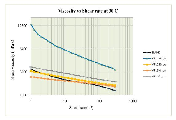
Figure (4-3): Viscosity Vs. Shear rate for sample (1) with different concentration at 30 C.
