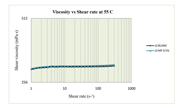
Figure (4-17): Viscosity Vs. Shear rate for sample (2) with 0.5% MF concentration at 55 C.
