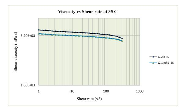
Figure (4-11): Viscosity Vs. Shear rate for sample (2) with 0.5% MF concentration at 35 C.
