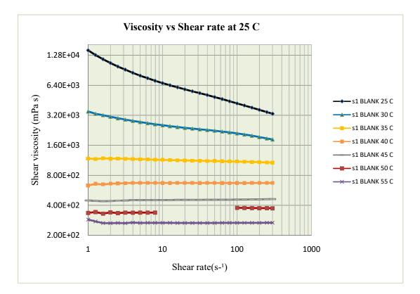
Figure (4-1): Viscosity Vs. Shear rate for sample (1) with different temperature.
