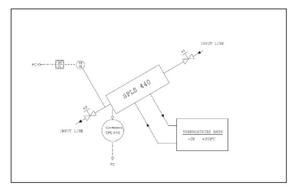
Figure (3-8): Schematic of electromagnetic viscometer diagram.
