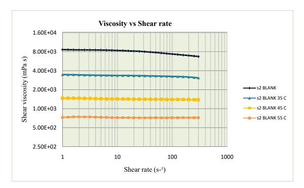
Figure (4-9): Viscosity Vs. Shear rate for sample (2) with different temperature.
