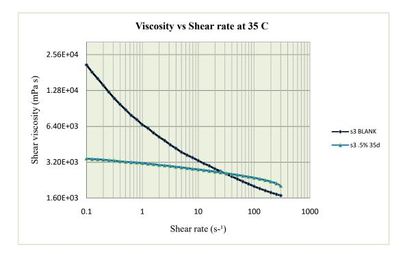
Figure (4-15): Viscosity Vs. Shear rate for sample (3) with 0.5% MF concentration at 35 C.
