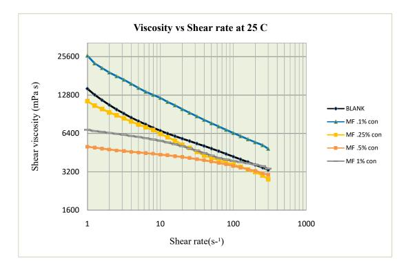
Figure (4-2): Viscosity Vs. Shear rate for sample (1) with different concentration at 25 C.
