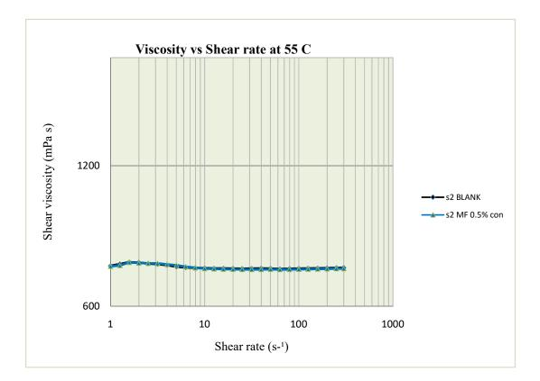
Figure (4-13): Viscosity Vs. Shear rate for sample (2) with 0.5% MF concentration at 55C.
