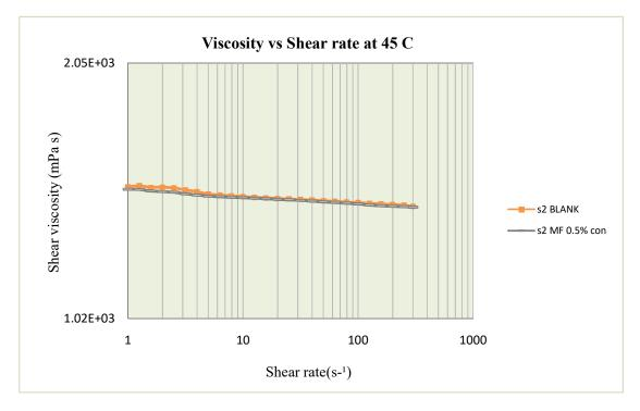
Figure (4-12): Viscosity Vs. Shear rate for sample (2) with 0.5% MF concentration at 45C.
