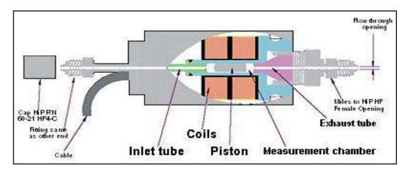
Figure (3-9): parts of chamber.
