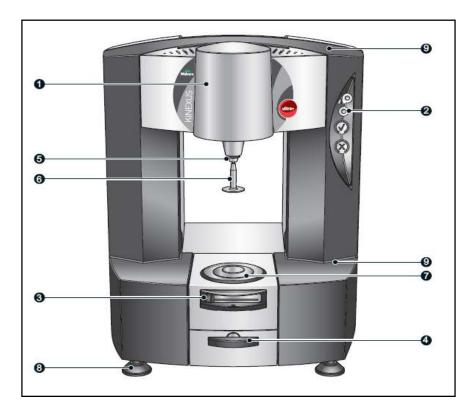
Figure (3- 6): Front view of Kinexus Pro apparatous.
