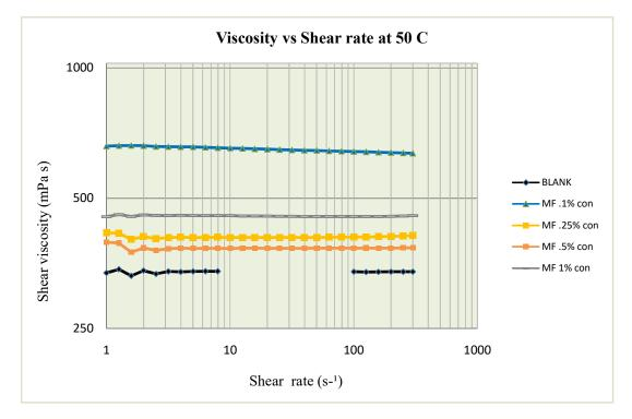
Figure (4-7): Viscosity Vs. Shear rate for sample (1) with different concentration at 50 C.
