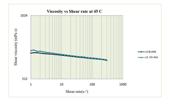
Figure (4-16): Viscosity Vs. Shear rate for sample (2) with 0.5% MF concentration at 45 C.
