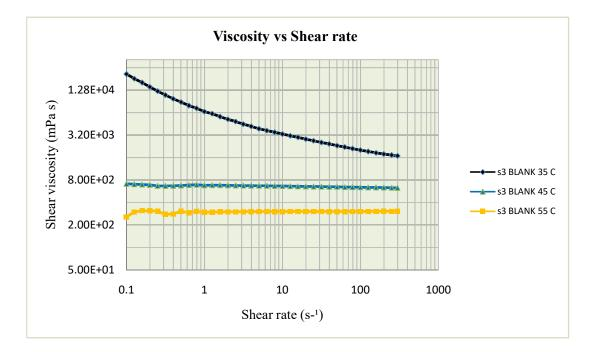
Figure (4-14): Viscosity Vs. Shear rate for sample (3) with different temperature.
