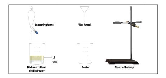
Figure (3- 5): Material required for oil-water separation process.
