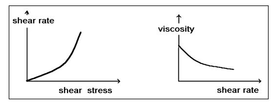
Figure (2-2): Pseudo plastic fluid, displays relationship between shear stress and shear rate and the fluid's viscosity at a varying shear rate. (rheo, 2014)
