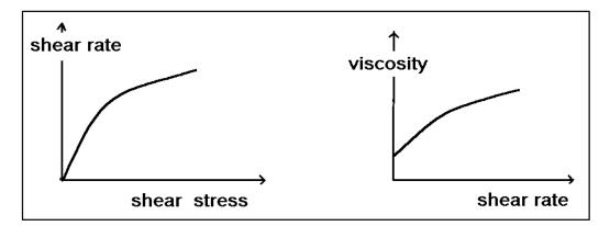
Figure (2-3): Dilatant displays relationship between shear stress and shear rate and the fluid's viscosity at a varying shear rate. (rheo.html, 2014)
