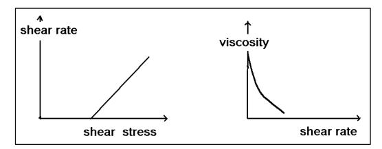
Figure (2- 4): Bingham displays relationship between shear stress and shear rate and the fluid's viscosity at a varying shear rate. (rheo.html, 2014)
