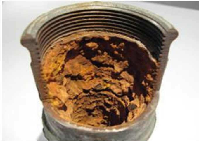
Figure (2.7): Formation of Scale in the Pipe(Theyab, 2018).
