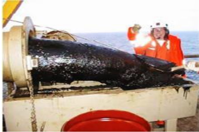
Figure (2.3): Wax Deposition Plug in the Wellbore On Platform C in the North Sea(Akpabio, 2013).
