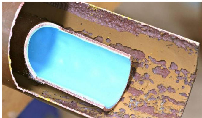
Figure (2.10): Erosion Formation in the Pipe(Theyab, 2018).
