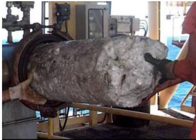
Figure (2.1): Hydrate Plug Formed in a Subsea Hydrocarbon Pipeline(Chaudhari, 2016, Bauck, 2013).
