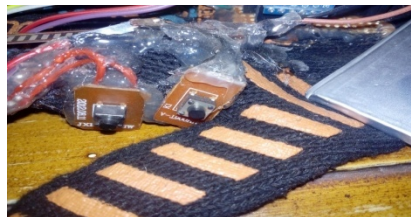
Figure 4.5: Installation Arduino Nano and Two pushbuttons
