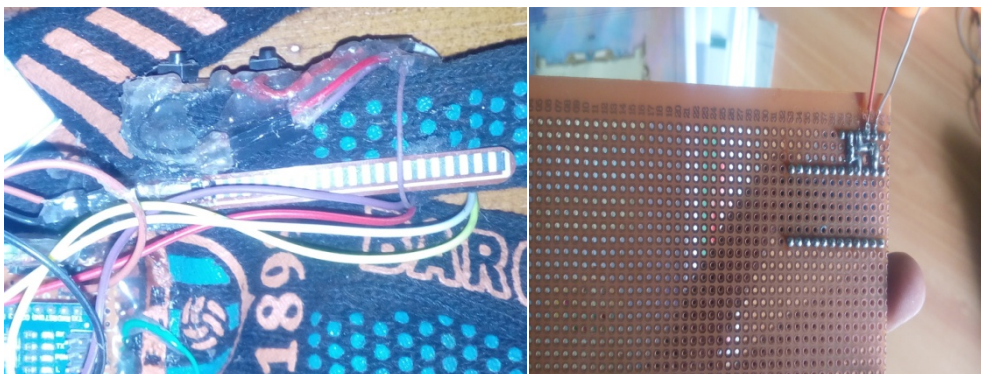
Figure 4.3: Installation Arduino Nano and Flex sensor
