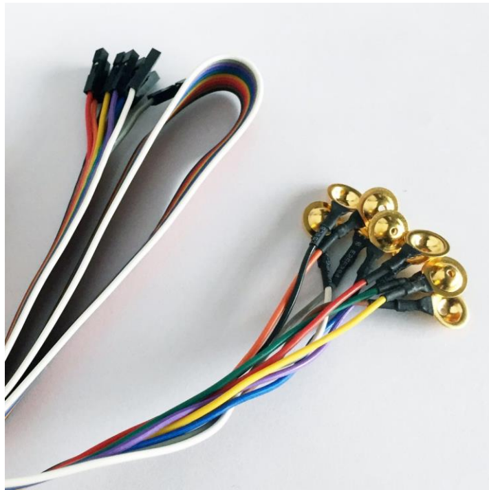
Figure (3.7): Gold Cup Electrode
