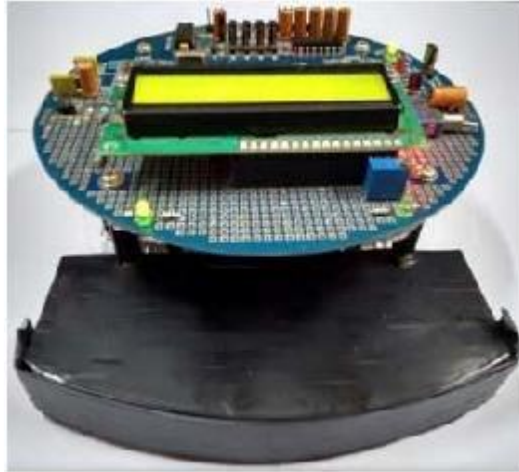
Figure 2.24: Two wheeled PID line follower using Arduino.
