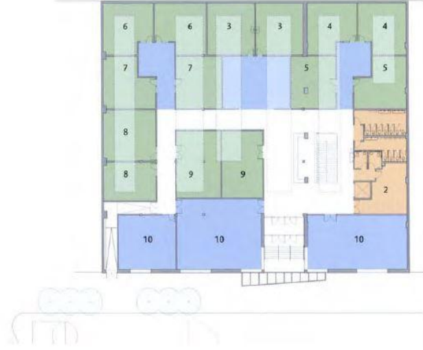
Ground floor plan 1 Multi-purpose room 2 Offices and storage 3 Kindergarten 4 First grade classroom 5 Second grade classroom 6 Third grade classroom 7 Fourth grade classroom 8 Fifth grade classroom 9 Sixth grade classroom 10 Music, dance and art spaces
