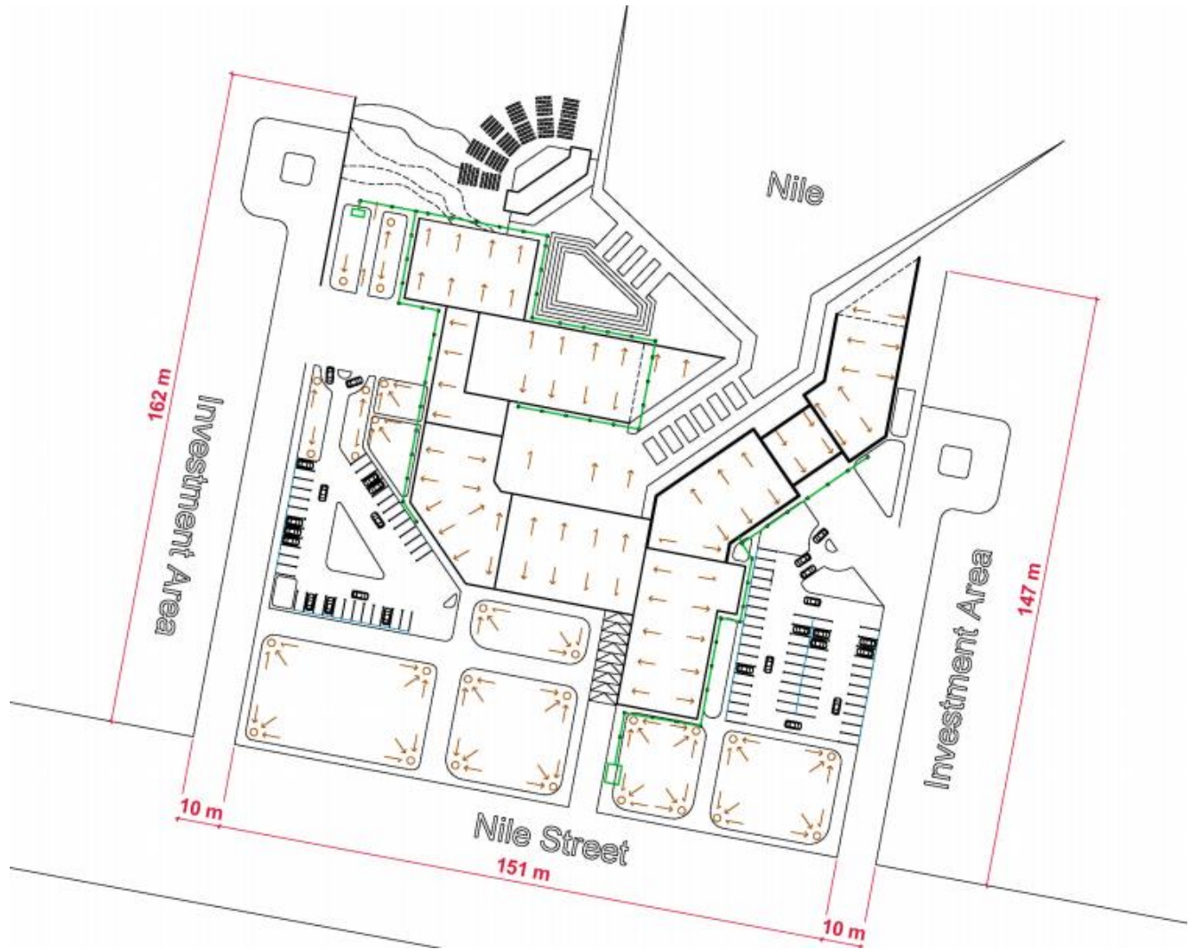
Figure 65: Site Plan showcasing how the sewage system and the drainage system are working
