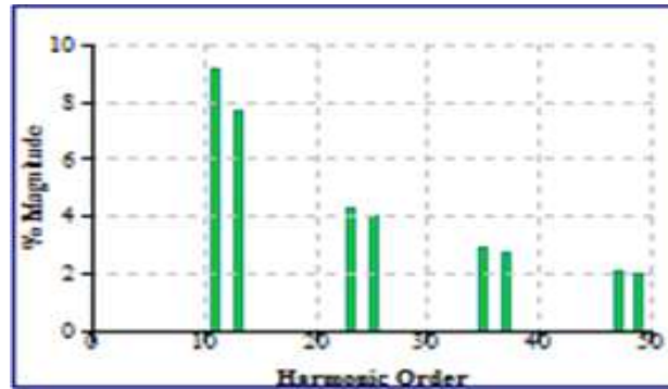
Figure 3.4 : Harmonic Source Spectrum for UPS
