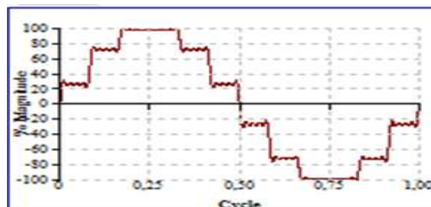
Figure 3.3: Harmonic Source waveform for UPS
