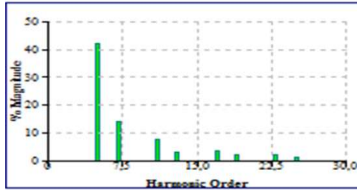
Figure 3.2 : Harmonic Source Spectrum for VFD
