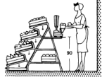
8 Counter with stands for boxes and baskets, drip pan and dirt trap
