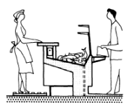
2 Fish counter with cooling compartment and drain
