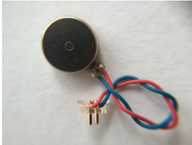
Figure 3.4: vibration motor (coin type)
