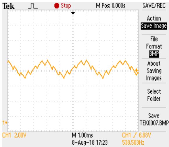
Figure 16: Measured voltage waveforms for two level VSI after filter
