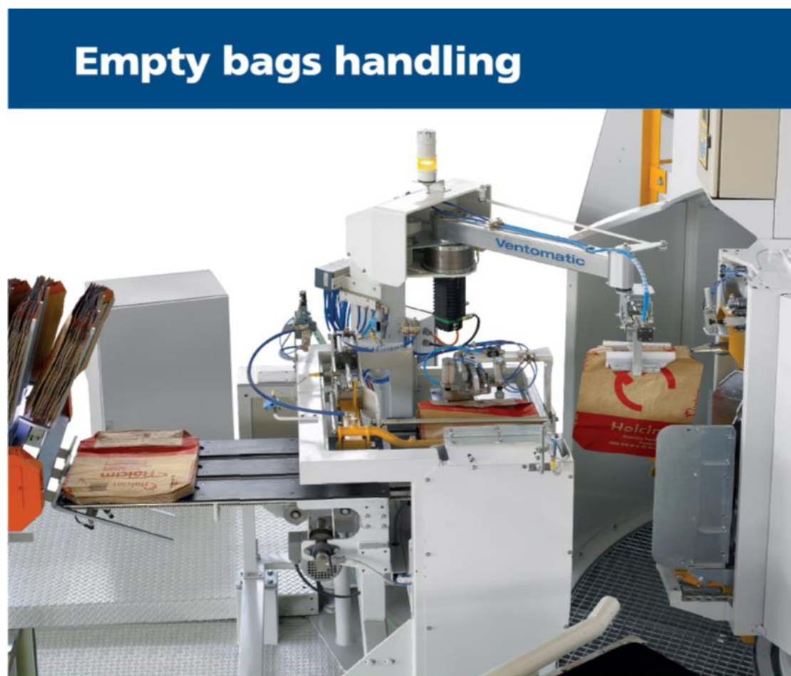
Figure (3.5) Bag applicator arm fixed the bag
