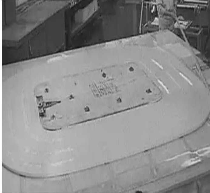
Figure 2.2: Pancake winding during winding process
