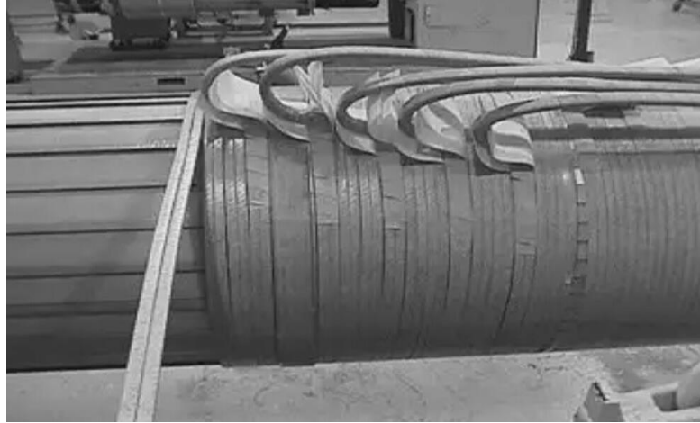
Figure 2.4: Layer windings (single layer with two strands wound in parallel)
